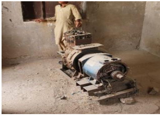
Old diesel engine was used to pul water from dug well in village Bhadasanda
